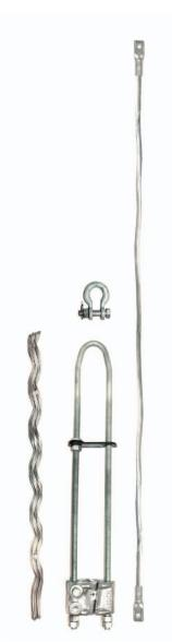
The Fiberlign Deadend is designed to terminate Optical Ground Wire (OPGW) while minimising any compression stresses that may be transferred to the core or optical elements within. The combination of retaining rods, wedge and housing distribute axial and compressive loading over a large area of the OPGW cable. Left-hand or right-hand lay style is provided to suit left-hand or right-hand lay OPGW respectively.
